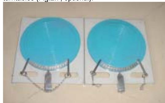
Fig.2.6 mechanical turntables
