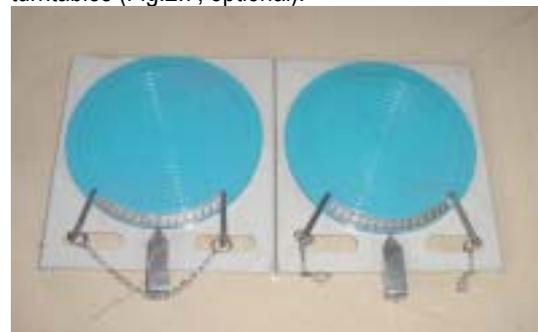
Fig.2.6 mechanical turntables
