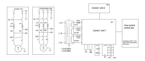
KM-Contactor; M-Motor; QC-Power switch; T-Transformer; SB1-UP button; SB4-STOP button; YA1 \ YA2 \ YA3 \ Y4-Electromagnet YV-Solenoid valve; SQ-Limit switch; XS-Socket of light; FU-Fuse
